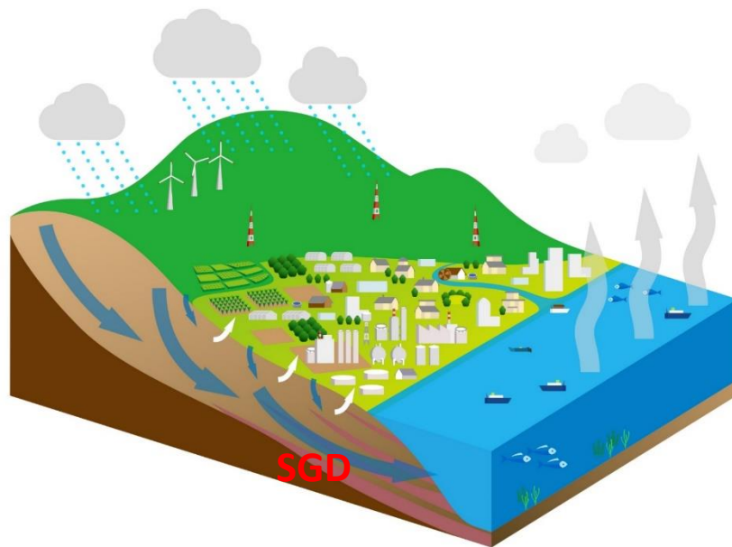
Figure 4. Schematic of Submarine Groundwater Discharge (SGD) (courtesy of the RIHN W-E-F- Nexus project).
